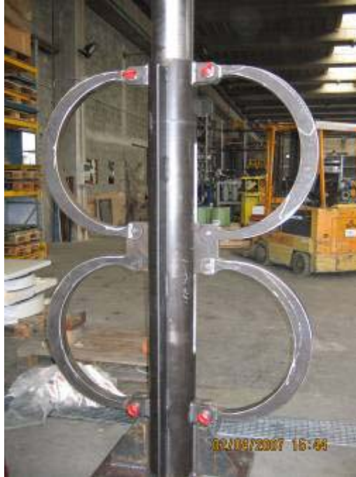
Figure 9 Steel frame and hysteretic C-shape dissipators for the laboratory test
