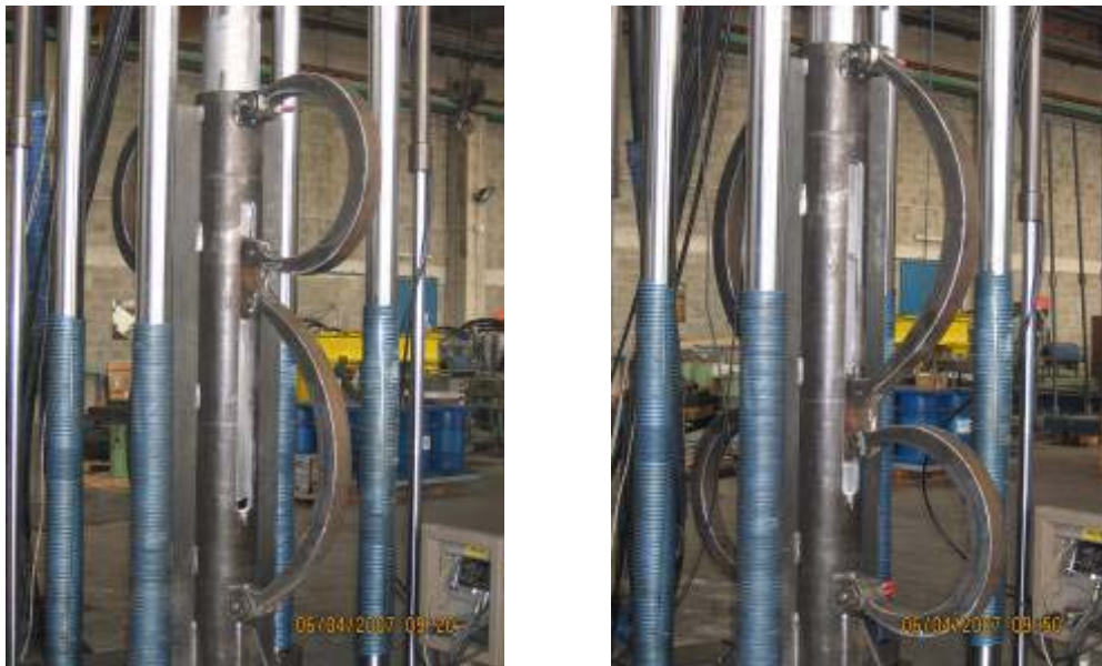
Figure 9 Steel frame and hysteretic C-shape dissipators for the laboratory test
