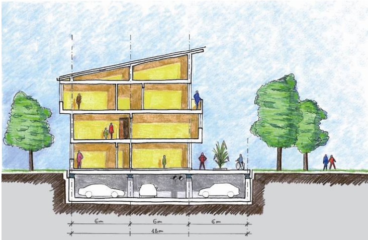
Fig. 2 – The conceptual design of the buildings for the C.A.S.E. project
