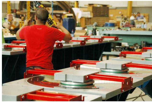
Figure 10 – The assembling line reached a peak of over 100 isolators per day
