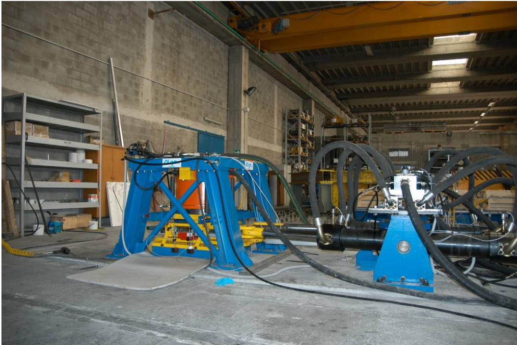
Fig. 11 – Dynamic testing equipment for sliding pendulum isolators at ALGA laboratory
